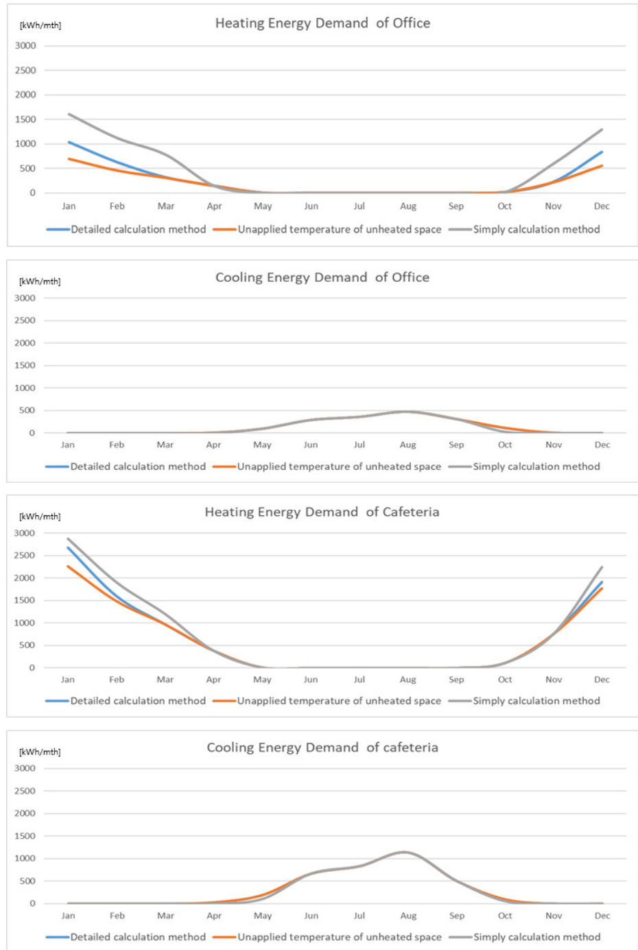
Figure 3. Energy demand results through detailed calculation method, unapplied temperature of unheated space, and simple calculation method
