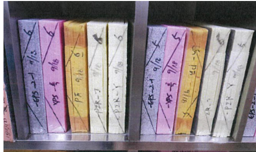
Figure 2. Specimens of the insulation materials for KS M ISO 11561
