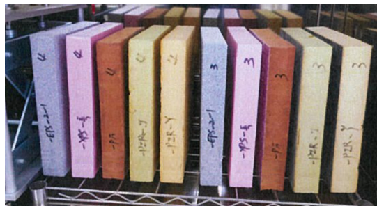
Figure 3. Specimens of the insulation materials for EN 13166 of the heat ageing method
