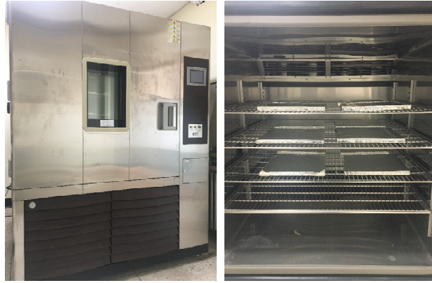
Figure 8. Constant temperature and humidity chamber for aging test of VIPs (left: exterior, right: inside of equipment)
