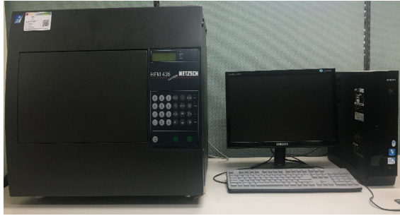
Figure 5. Thermal conductivity measuring equipment
