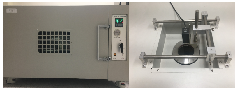
Figure 7. Inner pressure measuring equipment for VIP
